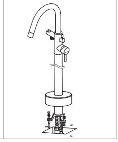
6. Insert the fixing bolts and fix tight in the floor. Move the cover to hide the base.
