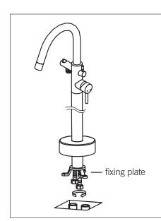
4.Insert the sliding cover on square pole, insert the flexible hose's nuts throw the fixing base and connect the G 1/2 nuts with the water net connectors fixing tight by key.
