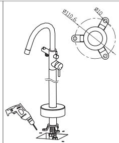
5. Adjust the complete to get correct position, then drill to fix base plate.
